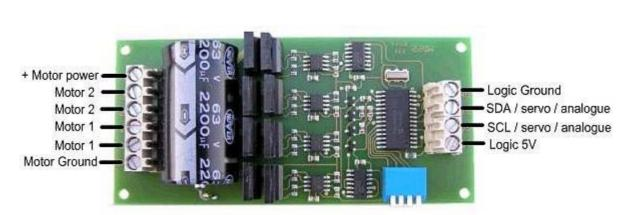
The Motor Ground and the Logic Ground are internally connected on the Module. Be sure to use cable rated for at least 10A for the Battery, Fuse and Motor leads.
