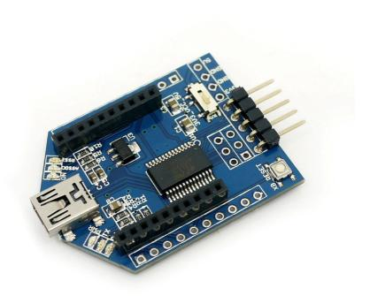
UartSBee V3.1 is a compact USB to serial adapter equipped with BEE (20pin 2.0mm) sockets. With integrated FT232 IC, It can be used for programming or communicating with MCU applications. On the other hand, you may connect your PC to various wireless applications via the BEE compatible modules.
