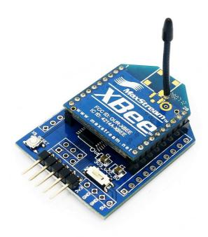
When BEE modules are plugged, it can either connect to PC via USB as wireless adapter, or connect to MCU via serial pins as wireless add-on. You may find BEE modules including Xbee, GPS Bee, RF Bee, Blue Bee, Wifi Bee and many other upcoming.
