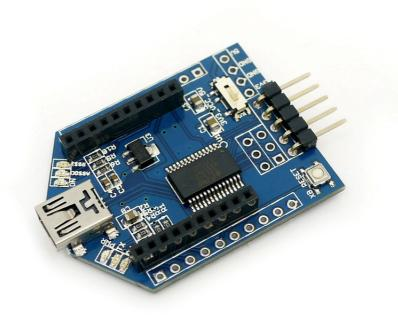
UartSBee V3.1 is a compact USB to serial adapter equipped with BEE (20pin 2.0mm) sockets. With integrated FT232 IC, It can be used for programming or communicating with MCU applications. On the other hand, you may connect your PC to various wireless applications via the BEE compatible modules.
