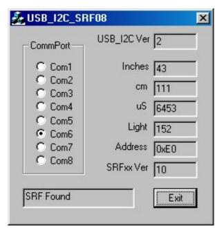
The connector on the USB-I2C module may be soldered directly to the SRF08 as shown, or you can use a cable if preferred. The USB-I2C module can easily supply the 25mA peak of the SRF08. The software automatically searches for the SRF08 and displays its I2C address, along with revision number, range and light sensor reading. You can download <u>usb\_i2c\_srf08.exe</u> and the <u>C source code</u> here.
