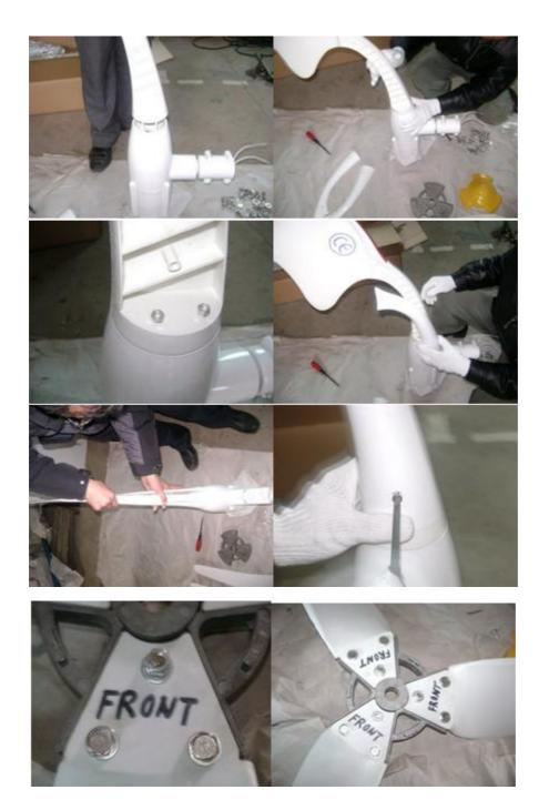
Note: when assembling the blades to the hub, please take care of the bolt position. 2 bolts shall go down the hub while one bolt comes up. Please see the picture
