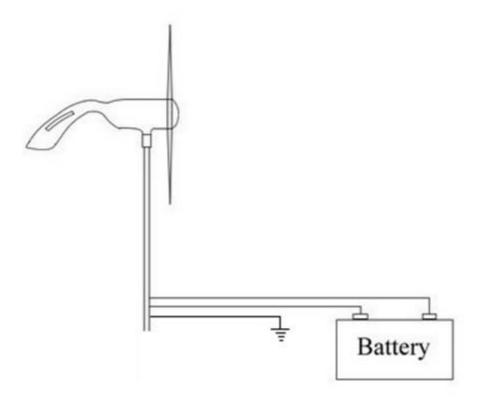
We recommend you wire the turbine directly to the battery bank to its own set of battery posts. This internal regulator will independently monitor the battery and charge as necessary.
