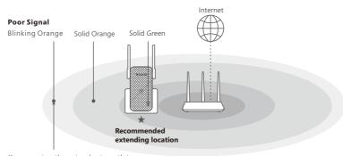
Keep moving the extender to outlets ser to the router until the LED indicator on the extender lights solid green.
