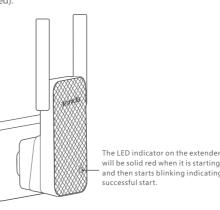
Relocate the extender to other electrical outlet. Observe the LED indicator on the extender to choose an optimum extended location for best WiFi performance.
