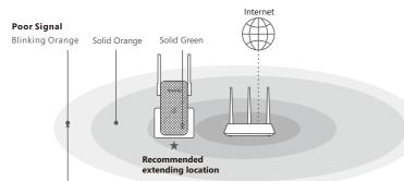
closer to the router until the LED indicator on the extender lights solid green.
