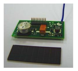
Figure 1: STM 11x sensor transmitter module
