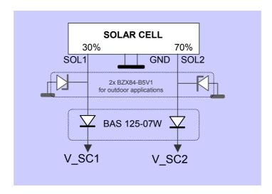
Figure 9: Connecting the solar cell
