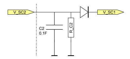
R\_C2: ~375 k $\Omega$  after 3 V applied for 10 min., ~5M $\Omega$  after 24h
