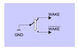
Figure 4: External WAKE pin circuit
