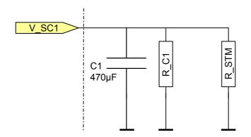
R\_C1: ~6 M $\Omega$  after 3 V applied for 10 min, >>10M $\Omega$  after 24h.
