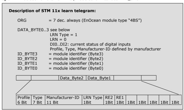
With this special learn telegram it is possible to identify the manufacturer of a device and the profile and type of a device. There is a list available describing the functionalities of the respective products. Please contact EnOcean to receive this list.
