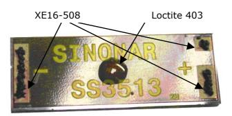
Figure 10: Gluing the solar cell
