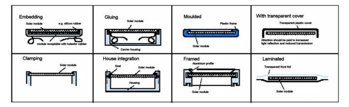
Figure 11: Examples of solar cell mounting
