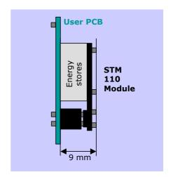
Figure 7: Examples of compact sensor unit
