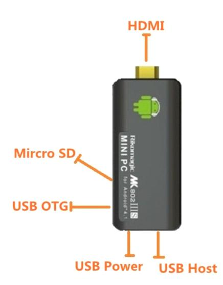
Micro-USB Power: Connect with TV USB port for charge the unit.
