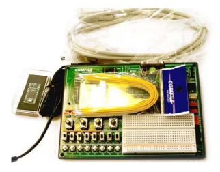
1) You should have received a module, study board, DC Jack, Yellow Jumper wires, serial cable, and a manual with your start kit.
