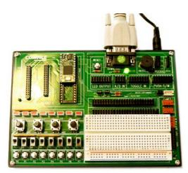
2) Simply put the CB220 into the DIP socket like shown in above picture. Connect the serial cable to the TOP serial port of the study board. You can connect 9-12V to the + and – of the DC Jack. The polarity does not matter for the study board, so simply hook + to one of the lines and – to the other. If you bought our 12V DC Adaptor, you can simply plug that in.
