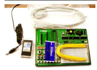
1) You should have received a module, study board, DC Jack, Yellow Jumper wires, serial cable, and a manual with your start kit.
