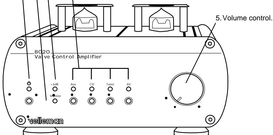
☞ The +6dB function can be used to adjust the level between the different sources. That way, when switching over between sources the volume will approximately remain the same.
