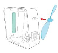
Remove the fan blade from the box. Push the blade onto the axis of the motor slowly and carefully.
