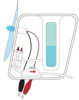
Open the purging valve by pushing the switch to the right side.
