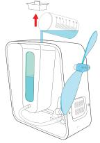
Pour the solution into the ethanol container. Put the lid back to the container.
