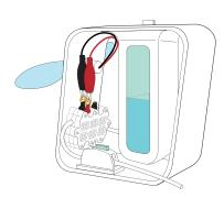
After waiting for 5-10 minutes, connect the two crocodile clips that are attached to the motor to the two terminal plates of the fuel cells current collector, which are both located on the upper part of the fuel cell.
