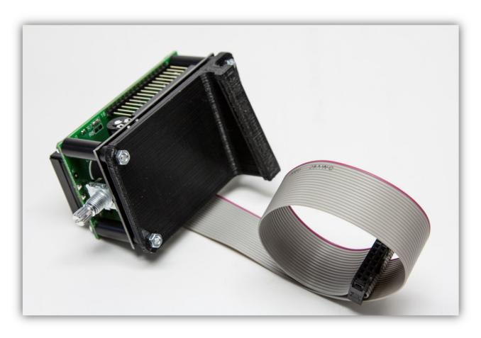
Snap the front of the enclosure to the module.
