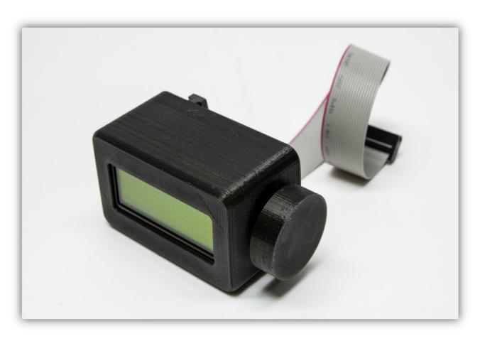
Slide the module down the groove of the right aluminium post. You will have to loosen the spool mount and remove some tie strips. It is possible that you will have to sand the clip on the back of the enclosure a bit so it will slide down easily.
