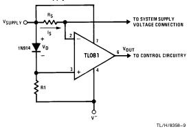
$\bullet~V_{OUT}$  switches high when  $R_SI_S>V_D$
