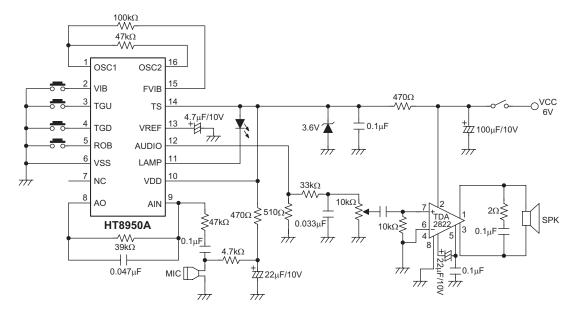
18-Pin Version with a TDA2822 Power Amplifier and a 6V Power Supply
