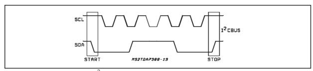
Figure 5: Acknowledge on the I<sup>2</sup>CBUS
