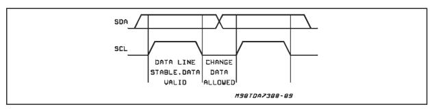
Figure 4: Timing Diagram of I<sup>2</sup>CBUS
