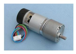
The EGM30 (encoder, motor, gearbox 30:1) is a 12v motor fully equipped with encoders and a 30:1 reduction gearbox. It is ideal for small or medium robotic applications, providing cost effective drive and feedback for the user. It also includes a standard noise suppression capacitor across the motor windings.
