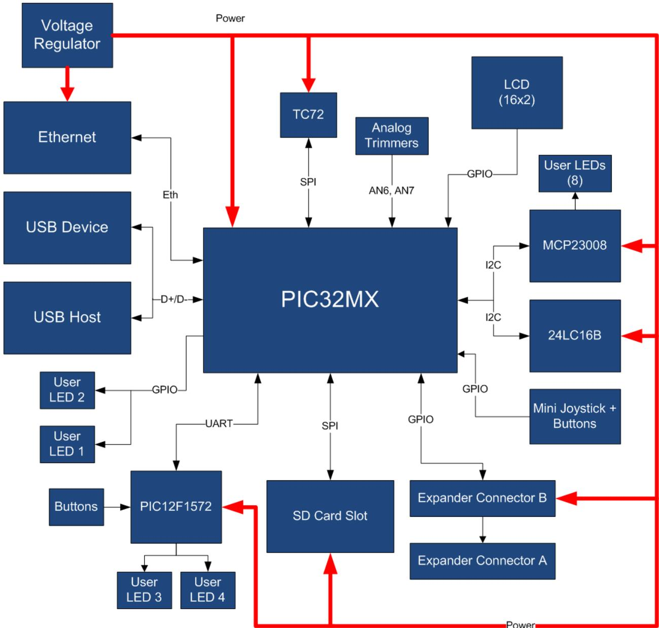
Figure 1 - Block Diagram
