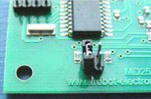
Serial mode at 19200 bps, 1 start bit, 2 stop bits, no parity
