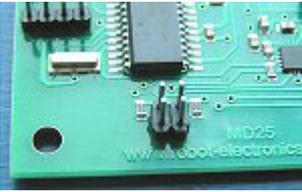
I2C mode with no jumpers installed, up to 100 khz clock
