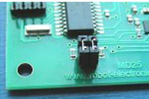
Serial mode at 38400 bps, 1 start bit, 2 stop bits, no parity
