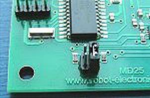
Serial mode at 9600 bps, 1 start bit, 2 stop bits, no parity
