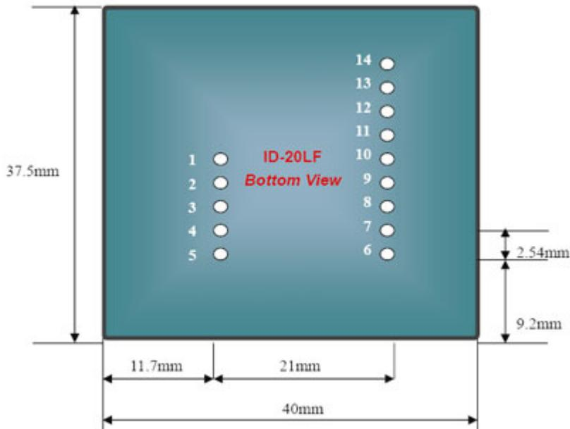
1. Zero Volts and tuning Capacitor Ground
