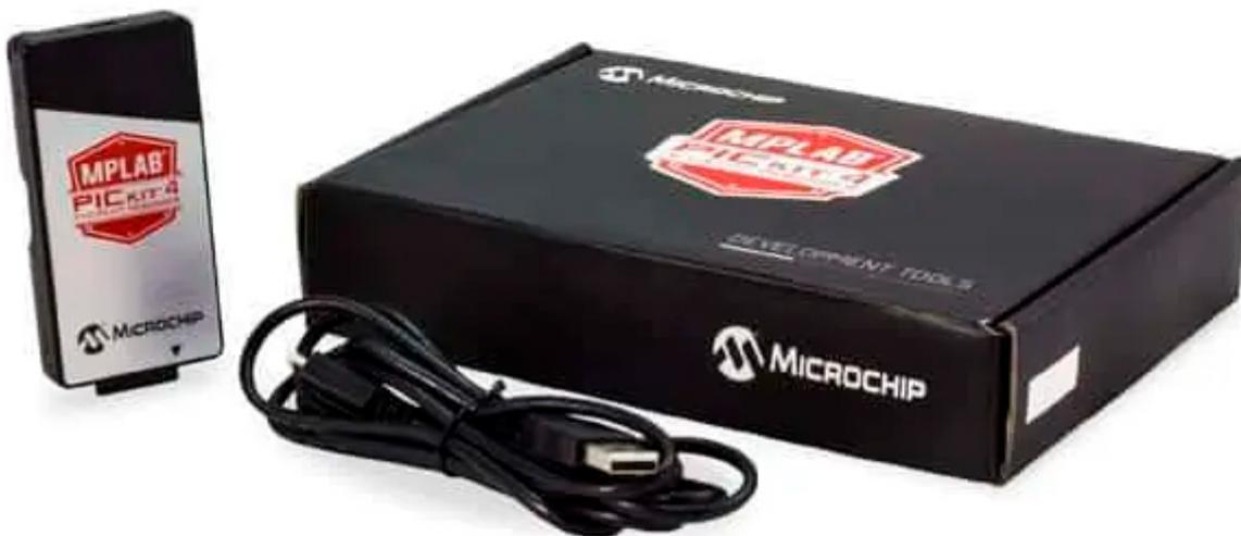
**MPLAB® PICKit 4 In-Circuit Debugger**
