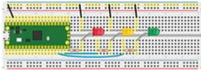
Figure 9-1: A basic three-light traffic light system
