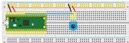
Figure 9-2: Wiring the potentiometer as a voltage divider
