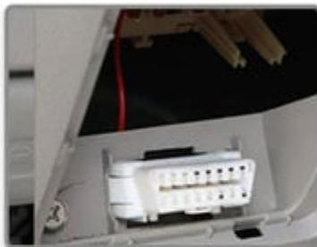
**2** Plug in the adapter into the OBD Port
